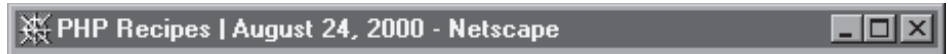
Figure 1-2. A simple PHP function, date() , formats the date for display in the browser title bar.
